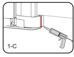
Silicone inside of the vertical slot before fitting the bottom seal strip.
