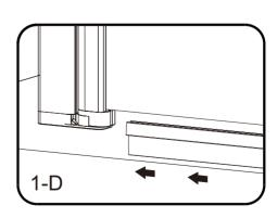
Insert bottom blade onto the glass and into the pre siliconed slot.
